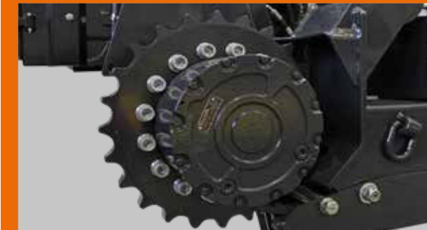
Cogwheel of the tracks in tempered steel
