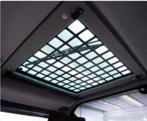
Roof window with safety grill, sunshade and windshield wiper
